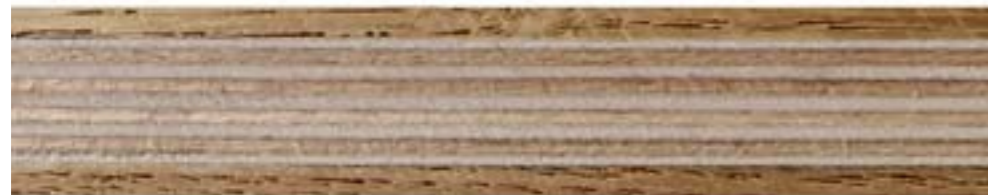
Hardwood with plywood core
