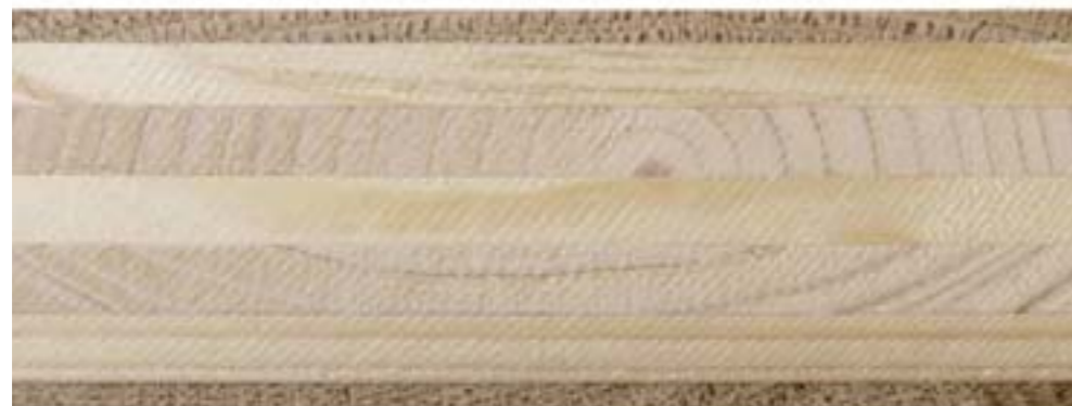
Hardwood with softwood core in 5 layers
